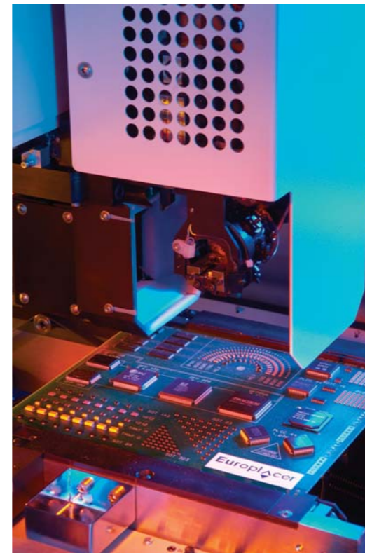
Placement head(s) are fitted with rotary turret head(s) with 8 or 12 pick ups.
