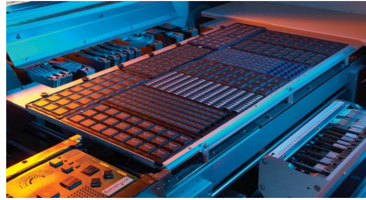
Huge area for 10 Jeduc trays on the single head machine, without reducing the feeder capacity
