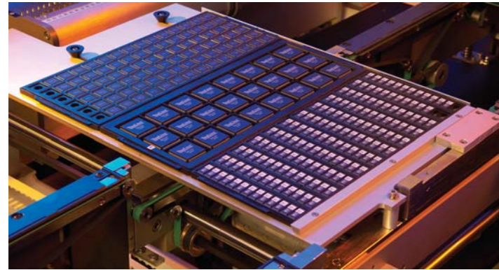
Area for 3 Jeduc trays on the dual heads machine, without reducing the feeder capacity
