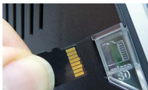
Micro smart SD card for parameterization of the i-CON PICO
